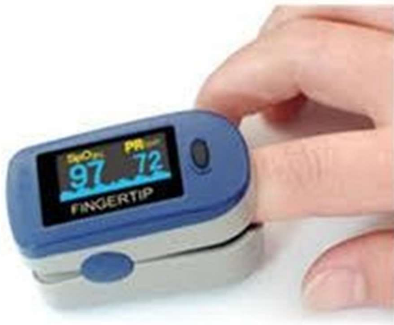
PulseOx- Measure pulse and oxygen saturation
